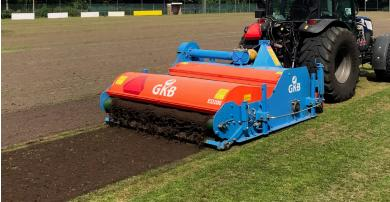
The Ecodresser is available in 4 different widths. This varies from 1.30m to 2.40m. The ED200 and ED240 are optionally available with a stone sieve. This prevents small excavated stones from ending up on the field. The ED130 and ED160 are supplied without a conveyor belt as standard. This is optionally available to guarantee a better distribution of the dress soil.
