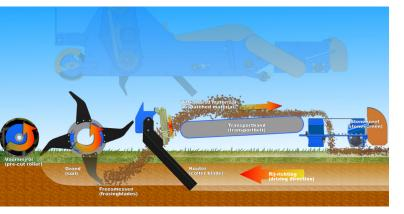
Depending on the version, the Ecodresser makes 4 to 7 slots in the field from which it extracts the dressing soil. The soil is then thrown onto the conveyor belt and then evenly distributed on the field. The coulters sit between the milling cutters and close the slots again. In addition to top dressing, the Ecodresser also has an aerating effect, with 9 to 15 slots per working width!
