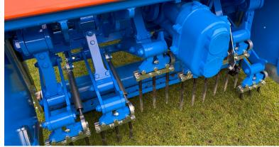
The Deep Tine Aerator features 6 - 10 arms that feature a unique tine mounting system. This allows you to quickly change the tines, which makes your work as a field manager or greenkeeper easier. Different types of tine holders and tines are available for the Deep Tine Aerator. This way the Deep Tine Aerator can be precisely adjusted for every challenge you have!
