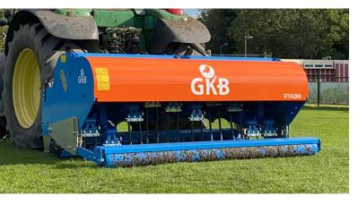
The DTA is available in four different versions. From the DTA120, with a working width of 120 cm and a maximum working depth of 25 cm, to the DTA260, with a working width of 260 cm and a maximum working depth of 40 cm. With the help of the pry angle adjustment of up to 25 degrees, you can choose to aerate your field even more intensively. The DTA210 and DTA260 are hydraulically adjustable in height.
