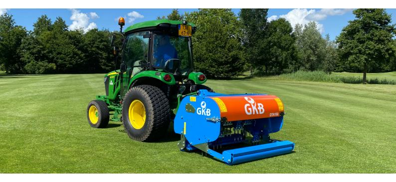
A compact top layer is a problem that affects field managers and greenkeepers worldwide. With the GKB Deep Tine Aerator, these problems are a thing of the past. The Deep Tine Aerator penetrates deep into the compacted turf, making the roots accessible to water and air again. The desired hole pattern can be created by means of a heavy-duty three-speed gearbox. Not only the gearbox is heavy-duty; the Deep Tine Aerator is designed with thick steel plates, making it suitable for any job!
