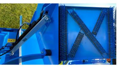
We deliver the brush with two extra side-decks as standard. Accordingly, you are able to broaden the operating width to as much as 4 metres. Consequently, you can move to the next pitch twice as fast. Because you can hydraulically fold the side-decks, you can also quickly go from one pitch to another. Have you finished your operation? Then you can put the Brush in the park position to protect your brushes, ready for the next challenge.
