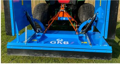
The Brush essentially consists of a 2 meter wide frame, under which stiff brushes are mounted. Under the deck, the brushes are located at the front and rear, as well as mounted diagonally. The positioning and stiffness of the brushes has been designed in such a way that infill is distributed as effectively as possible and the appearance of the fibers meets your expectations.
