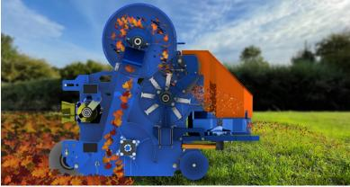
The built-in safety mechanism ensures that hard materials such as stones can leave the machine. After crushing in the hammer mill, the mulch is thrown onto the disc unit. The pulverized leaf is thus spread behind the machine. The outflow can optionally be directed to the left and to the right. In this way, walking paths can be protected and the Leafreducer can be used safely.
