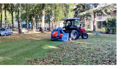
By pulverizing the leaves you also prevent suffocation of the lawn. This also contributes to the health of the grass. The Leafreducer picks up the leaf with the help of flails at the bottom of the machine, after which it is sucked further up by the turbine. The turbine ensures that the blade is reduced the first time. After this, the leaf is thrown into the hammer mill, where the leaf is ground into a fine mulch.
