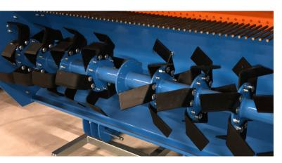
The Stoneburier can be equipped with 45° and 90° fraising blades. The 45° blades stir up the soil well, but result in a slightly messier working image. The 90° blades ensure a more even working image, but also press the soil a little more. In this way, there are always milling cutters available that meet your requirements. This ensures that the Stoneburier is a versatile machine that can be perfectly tailored to your challenge!
