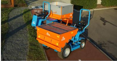
The most unique aspect of the Infiller is the rotating cab. In this way, spreading can take place in front of the machine, so that the infill is in the field before it is driven over. It is possible to partially tip the bunker while driving. This makes it possible to oversee the spreading quantity at the front of the machine. Everything to make your work as easy as possible!
