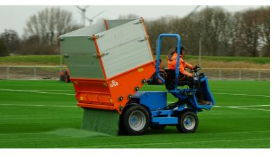
To regulate the amount of litter, the metering valve can be opened up to 100mm. Stirrers are present in the bunker to keep the material moving and to guarantee a smooth outflow. For safety, a collapsible grid is mounted on the Infiller. In addition, the Infiller is equipped with a travel lock, so that the machine cannot drive away unintentionally during adjustment. This way you can spread your field safely and efficiently.
