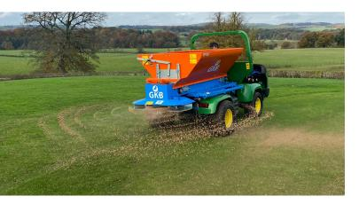
The SP100 comes in two versions. In addition to being available with a wheelset, it is also available as a superstructure for a Progator, Workman or Truckster. The SP100 is the largest mounted sand spreader on the market, with a flat-filled bunker capacity of  $1m^3/36$  ft<sup>3</sup>. The SP100 is built with a strong bunker and with the optional hydraulic control, this is the perfect machine for your sports field or golf course.
