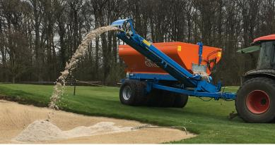
The SP230, SP300 and SP400 are GKB's larger sand spreaders, with a capacity of 2.3<sup>3</sup>, 3m<sup>3</sup> and 4m<sup>3</sup>. These are also available in an SPM variant. The SPM is a Sandspreader with a sand slide at both the front and the rear. At the front is a hydraulically operated elevator belt. This makes the SPM the ideal machine to refill machines such as the GKB Drainmaster. The SPM is also very suitable for filling sand bunkers and trenches.
