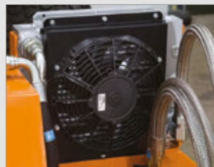
Integral heavy duty Oil cooler
