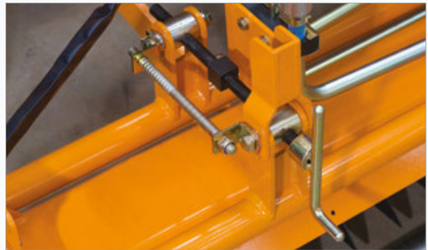
Micro adjusters for depth setting
