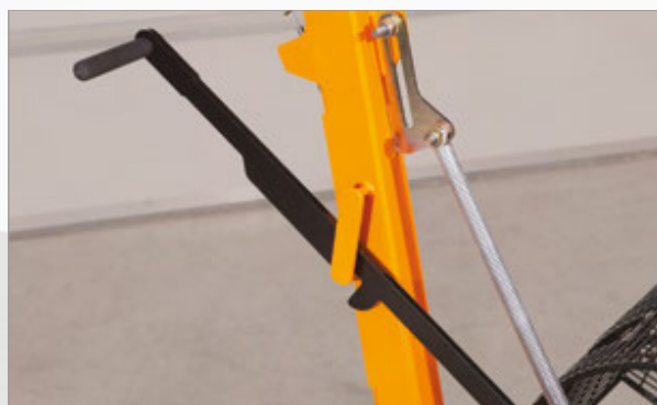
The cantilever system for lifting the machine out of operation
