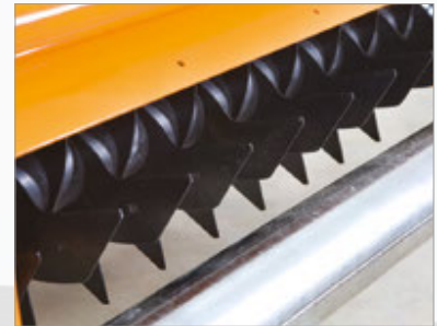
Tungsten tipped 'hook' blades for durability
