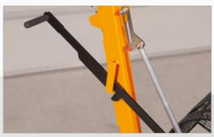
The cantilever system for lifting the machine out of operation
