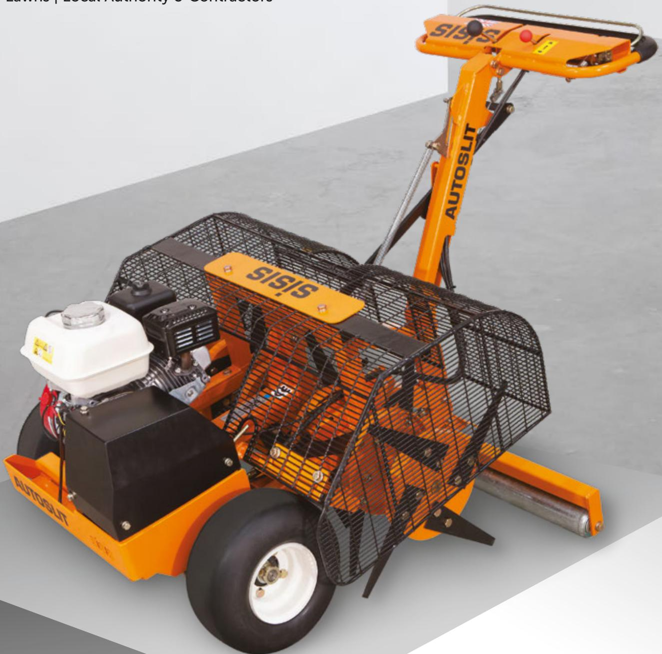
**A purpose built pedestrian deep slitter which is suitable for use on fine or outfield turf helping to reduce compaction and assist the percolation of surface water.**
