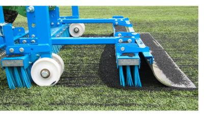
The Quick-Brush comes standard with two brushes, a rake, a height-adjustable wheel set and a rubber flap. Most tools can be separated from each other in order to adjust the Quick-Brush as well as possible to your field. This combination of working methods gives you a nice, even picture. In addition to the height adjustment, the wheels also ensure that the Quick-Brush leaves nice straight tracks.
