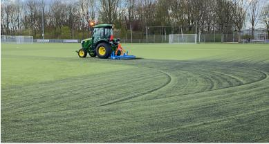
Regularly brushing the field prevents reduced drainage, deteriorated sports-technical properties due to hardening and the appearance of a polluted field. The brushed field regains the appearance it had on the day it was taken into use. With the Quick-Brush you always perform the right maintenance, whatever the requirements. This makes the Quick-Brush the ideal machine for your sports field!
