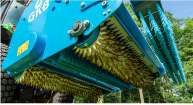
The Combiseeder can be fitted with conical spiked rollers or Cambridge discs. The spiked rollers create 1500 holes per square meter, after which the grass seed falls and is brushed into the holes. The second row of spiked rollers is slightly offset and closes the first row. As a result, the grass seed is buried, so that it cannot be eaten by birds or other animals.
