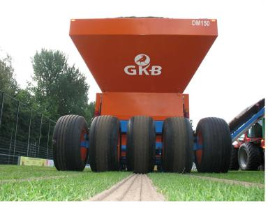
The Drainmaster is also available in a model with a working width of 85 cm. It creates two trenches instead of the three trenches that the DM150 creates. In addition, you can operate the DM850 with a tractor with at least 90 hp.
