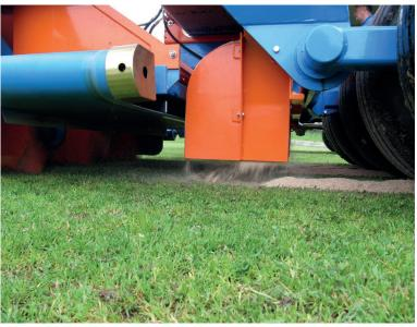
The trenches are filled with drainage sand to the operating depth of 23 cm during the same operation. The wheels of the Drainmaster will press the drainage sand into the trenches. The created drainage network ensures a higher playing capacity. Because of the strengthened grass, you will also experience less damage from the activities on the grass.
