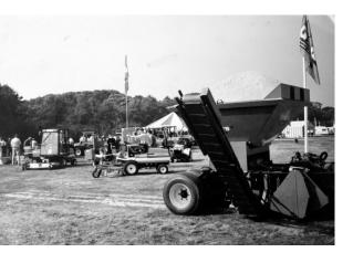
The GKB Drainmaster has been in continuous development since 1985. Throughout the years, the concept of the Drainmaster has constantly been refined. The Drainmaster was developed in order to improve and accelerate the drainage of surface water. Thereupon, the stability and quality of your grass will improve.
