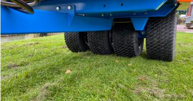
The Topdrop is equipped with four balloon tires for optimum ground pressure. The TD330 can optionally be equipped with a bumper with lighting and an overrun brake for use on public roads. The Topdrop is available in four different versions with different working widths and sand bunker capacity. This variation ensures that there is always a Topdrop that suits you!
