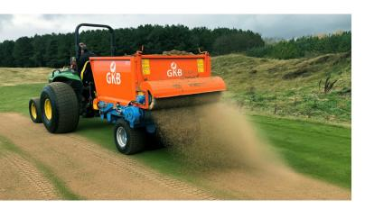
The material is transported to the metering valve by means of a conveyor belt. It is then spread behind the machine by the brush. Both the speed of the conveyor belt, the opening of the dosing valve and the position and speed of the brush can be adjusted, so that you can adjust the Topdrop exactly as you want it. This allows you to apply the material exactly in the right way and in the right place.
