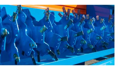
At the heart of the Vstrong is the rotor shaft, which can be fitted with the various scarifying blades. By using balancing weights, you can choose a center-to-center distance of 25, 50 or 75mm. The Vstrong is standard equipped with carbide 3mm scarifying blades. In combination with a counter-rotating direction, the Vstrong does not skip an inch.
