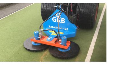
The Rotobrush is available in 2 versions. The RB040 is a single ø40 cm brush on a long arm. Optionally, a ø60 cm brush can be mounted. There is also the option to operate the RB040 hydraulically. In addition to the RB040, an RB120 is also available. This machine has 2 brushes of ø60 cm mounted and is adjusted in such a way that not even a centimeter is skipped.
