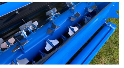
The VCollector is optimally equipped for weed removal thanks to the CombiRotor. This is a powered rotor developed for scarifying and milling. The rotor rotates against the direction of travel, so that it makes a powerful cutting movement and does not miss a centimetre. With the VCollector, the blades are mounted with wind vanes. This creates an air flow that sucks the milled material into the collection container.
