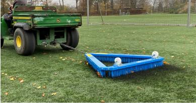
The Tbrush is suitable for brushing out different types of infill; think, for example, of rubber, sand and cork. Brushing the field regularly prevents reduced drainage, deteriorated sports-technical properties, such as hardening or the appearance of a polluted field. The brushed field regains the appearance it had on the day it was taken into use.
