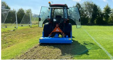
The unique aspect of the Renovator is the rotating brush heads. The 5 or 6 brush heads are packed in a compact machine, making the Renovator easy to work with. In addition, the machine can be used on both artificial and natural grass. This makes the Renovator the ideal machine to thoroughly improve your drainage or to make your turf healthy again.
