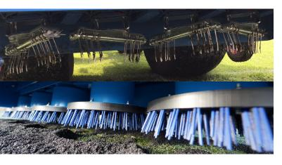
The Renovator is standard equipped with brushes for artificial grass. Optionally, it can be equipped with spring tines. The spring tines can be used on both artificial and natural grass. On artificial grass, the tines loosen the infill, while on natural grass they fight weeds. As a result, the Renovator mechanically ensures a healthy turf. This multifunctionality means that the Renovator can be used for various jobs.
