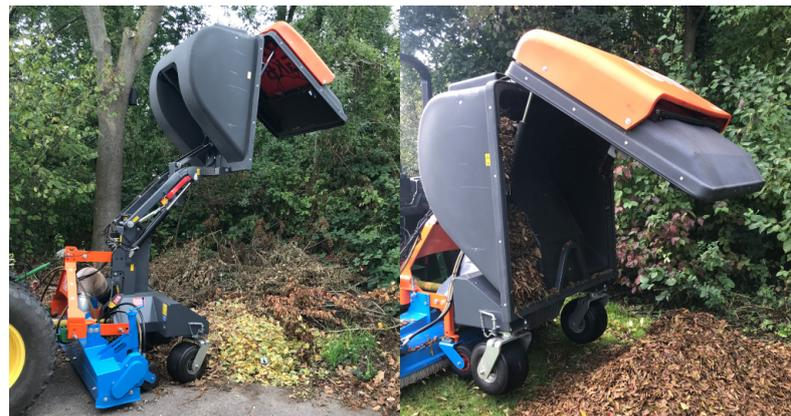
The fact that the Leaf-Clean leaves infill on the field, but does take the leaf with it, is due to a combination of a brush rotor and a suction mechanism. The brush rotor moves lightly over the artificial grass and takes the blade upwards. The Leaf-Clean's brush rotor and squeegee are fully adjustable, so it can be used on any type of infill. This makes the Leaf-Clean suitable for every artificial grass pitch!
