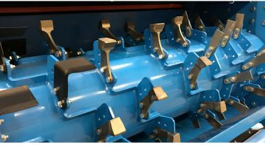
The Combinator is equipped with the GKB Combirotor®. This rotor can be provided with different types of blades for different operations. Because of this it is possible to mill and scarify with the same machine. In addition, there is also the possibility to equip the Combinator with a brushrotor. The brushrotor is used to efficiently remove the infill from your sports field.
